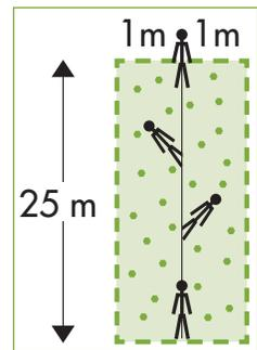
25 m measurement line and corresponding measurement area
